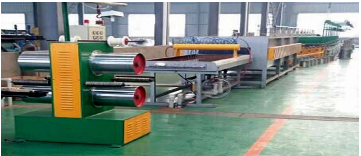
Four Roller Casters Machine with Cooling Water Tank - Annealing Furnace
