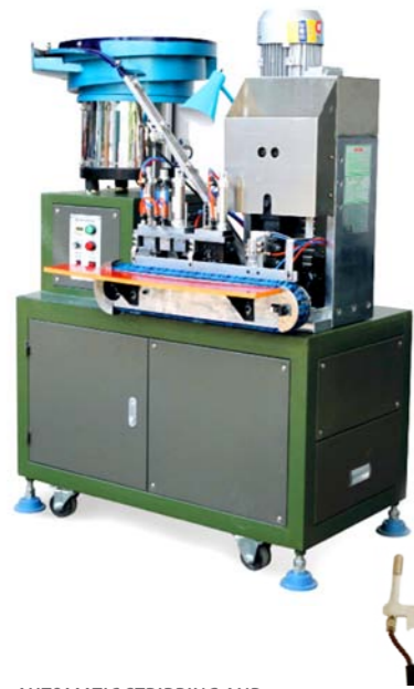
AUTOMATIC STRIPPING AND 2 PIN INSERT CRIMPING MACHINE
